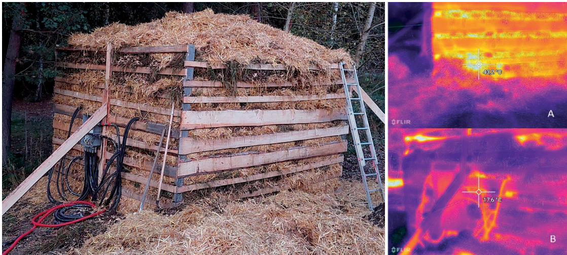
Fig. 1: Jean pain composting represents a low-cost method of heat production whereas a pile (4x4x4m) of type (B) biowaste can serve for family home or small business all winter long. The right section of the image shows an infrared image, where scan "A" indicates temperatures in the center of the pile (discharged to the house) are satisfactorily above 40°C and scan "B" indicates that after coming from the house heating circuit, the process fluid is returning at a temperature below 20°C.
