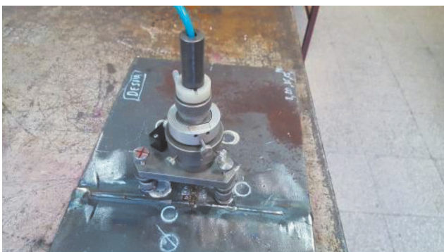
Fig. 4. Measurement of residual stresses
