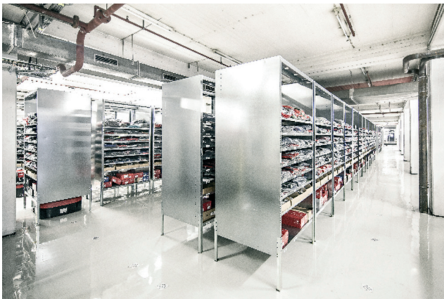
Fig. 1. SafeLog partner Swisslog's automated CarryPick system
