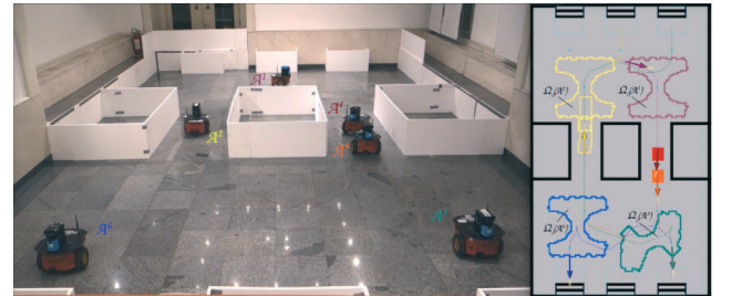
Fig. 6. Validation of the algorithm performance on a system composed of six Pioneer 3DX robots in a laboratory environment with terminals and corridors. [23].
