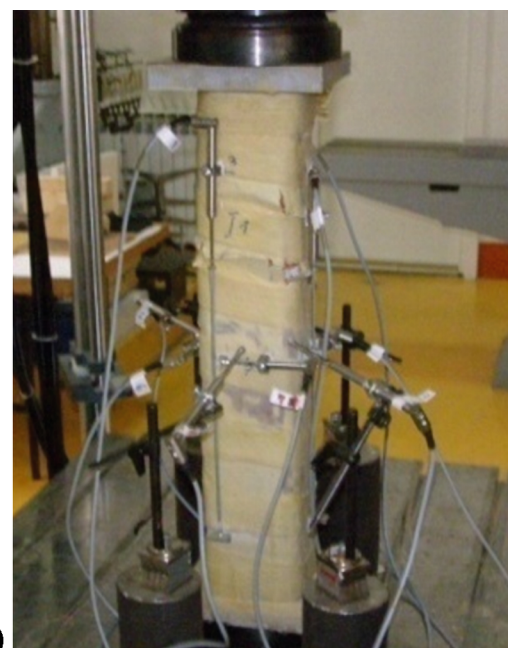
Fig. 4. a) Scheme of loading and LVDT setup and b) Specimen during testing
