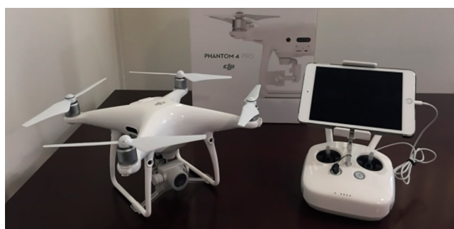
Fig. 4. UAS DJI Phantom 4 Pro with corresponding remote controller and tablet computer
