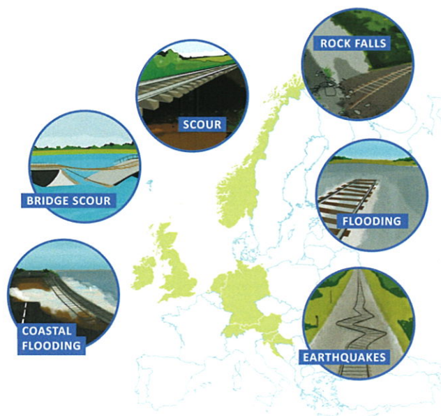
Fig. 1. Different types of failure on railway infrastructure [10]
