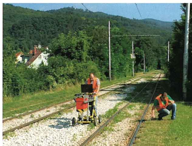
Fig. 7. Conduction of GPR investigations for the tram embankment condition assessment [10]
