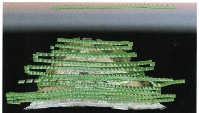
Fig. 21. Positions of 451 images taken from UAS
