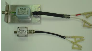
Figure 5. A photo of Mini-Circuits® FTB-1-6 (down) and North Hills™ 0300BA (up) transformers with cables and electrode clamps
