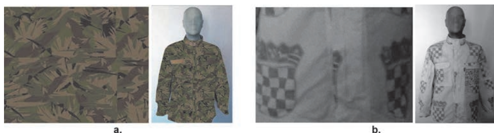
Figure 10: Military pattern with hidden message: 10a – image in VIS waveband (camouflage pattern); 10b – image in NIR waveband at 1000 nm (hidden message occurs, invisible to a naked eye in VIS waveband).
