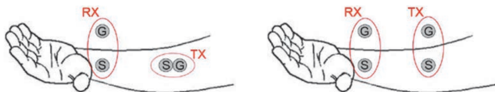
Fig. 8. – Positions of the electrodes: longitudinal direction (left), two-electrode arrangement (right).
