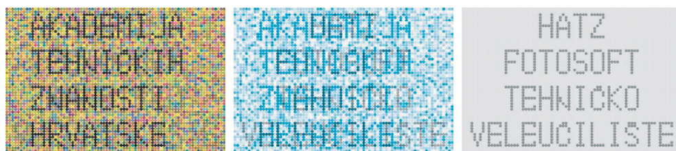
Fig. 2 a,b,c – Multicolored graphics in barijerma: V (400-700nm), 715 nm, 1000 nm
