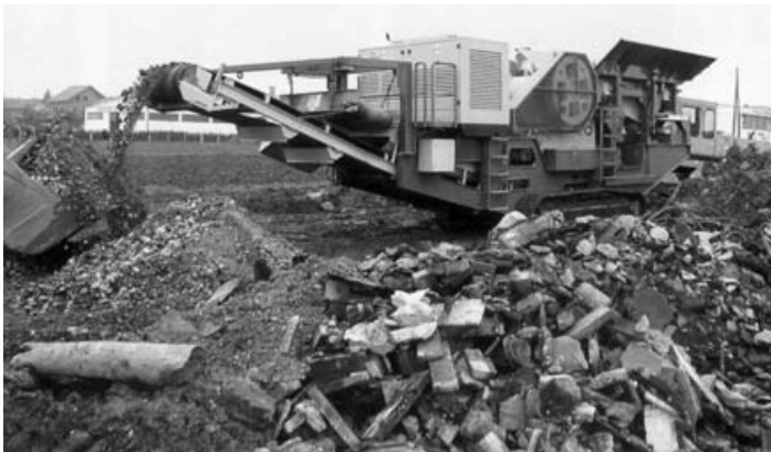
Figure 7: Mobile rubble crushing installation with crushing and screening unit
