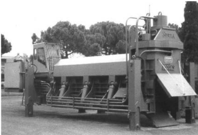
Figure 4: Hydraulic guillotine shear (Sierra Europe Recycling Ltd)
