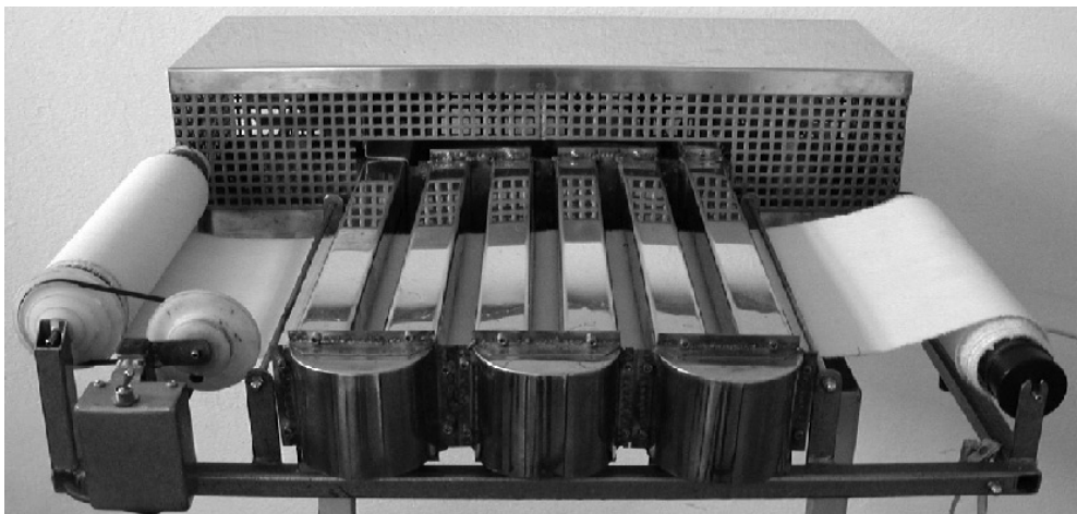
Figure 1: Planar microwave device constructed at Faculty of Textile Technology
