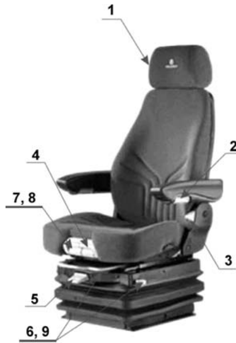
Figure 9. Tractor seat Grammer- ACTIMO XXL 12. 1 – Adjustable headrest, 2 – Foldable armrests adjustable height and angle, 3 – Adjustable seatback, 4 – Adjustable seat angle, 5 – Height adjustment, 6 – Fore/aft adjustment, 7 – Variable seat length, 8 – Adjustable airbag, 9 – longitudinal muffler
